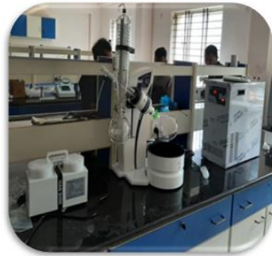
ROTARY EVAPORATOR WITH CHILLER AND VACUUM PUMP
