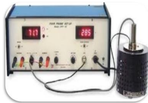
FOUR PROBE WITH HEATING OVEN
